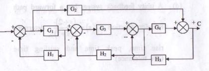
(c) Draw the signal Flow Graph and determine the overall transfer Function of the block diagram shown below.
